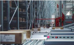
Automated light goods storage with Tornado miniload cranes Swisslog's Tornado miniload cranes uniquely combine high throughput, energy-efficient operation, and unmatched reliability.
